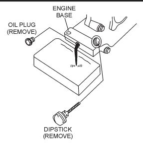
Figure 14. Engine Oil Plug
